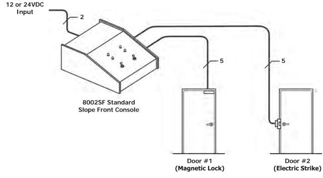
Doors require door status switch or lock status sensor for LED indicator monitoring.
