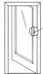
Device must seat flush on door surface or on shims that keep it parallel to door face.
