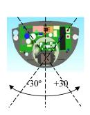
Sensing field as close to the door as possible: -antenna set at the position of **0**°
