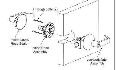
CAUTION: All fasteners in step 4 must be present and securely tightened to ensure proper functioning of lock. Loose or missing fasteners will lessen the safety, security and performance of lock.
