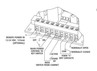
NOTE: "DC IN" are the only polarity sensitive terminals. When external power is used, battery will act as a backup. "Dry Contacts: NC, COM, NO" are used for remote alarm monitoring.
