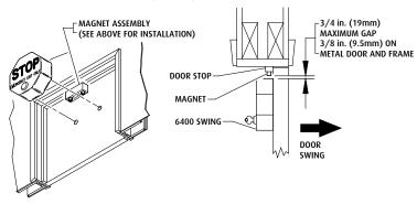
\*Note: When mounting reed switch on door and the main unit on wall, wire service loop must be used.
