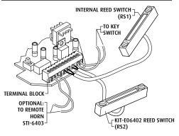
VIEW SHOWING INSTALLATION OF ADDTIONAL REED SWITCH KIT-E06402
