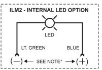
\*NOTE: ILM OPTION VOLTAGE \_\_\_\_\_ 12VDC \_\_\_\_ 24VDC
