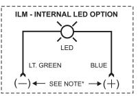
\*NOTE: ILM OPTION VOLTAGE 12VDC 24VDC
