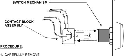
2. REMOVE THE PLUG-IN LAMP FROM THE SOCKET ON THE FRONT OF THE CONTACT BLOCK ASSEMBLY.
