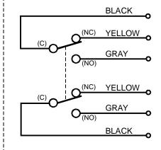
**DPDT ALTERNATE-ACTION CONTACTS RATED** 6 AMPS @ 125VAC
