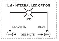
\*NOTE: ILM OPTION VOLTAGE \_\_\_\_ 12VDC \_\_\_\_ 24VDC
