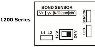
A terminal block is provided for wiring the maglock to the power supply and for the Bond Sensor Relay outputs. A pair of flying leads are provided for the Door Status Sensor (Reed Switch). These are the Green and White wires. It may be necessary to lift up the board to get to the Green and White wires.
