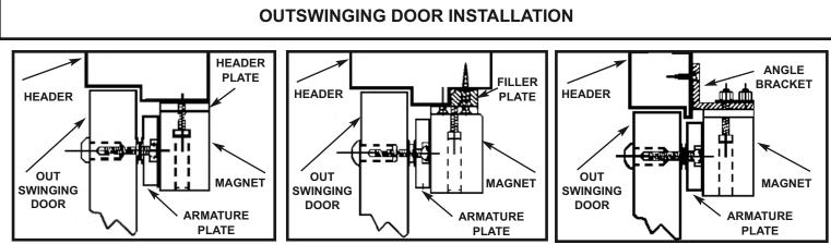
2. FOLD TEMPLATE ON DOTTED LINE TO FORM A 90 DEGREE ANGLE. TAPE TEMPLATE AGAINST DOOR HEADER WITH DOOR IN A CLOSED POSITION 1" FROM DOOR FRAME OPPOSITE HINGE SIDE OF DOOR JAMB. FOR A PAIR OF DOUBLE DOORS PLACE TEMPLATE AT THE CENTER OF THE DOOR OPENING. TRANSFER HOLE LOCATIONS TO DOOR AND FRAME HEADER, (SEE TEMPLATE INSTRUCTIONS).
