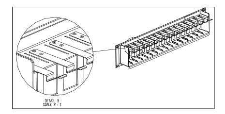
4. The baluns may be installed either front or rear facing. In order to remove each balun, lift the spring retaining clip at the rear of the chassis and pull out the balun in a horizontal direction.
