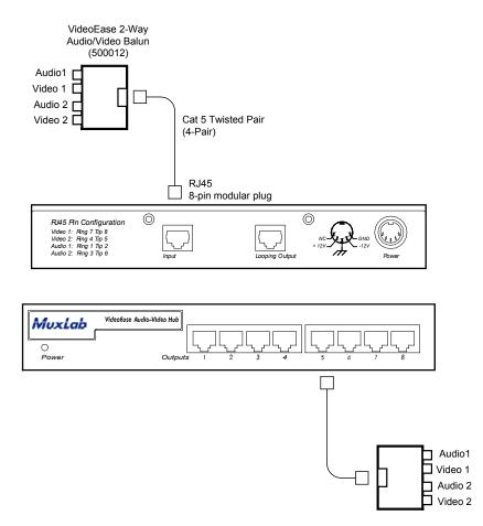
Figure 5 : Connection Diagram
