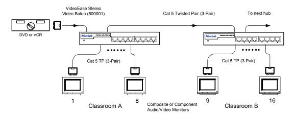
In order to cascade the first hub to a second hub, prepare a 4-pair Cat 5 cable from the Looping Output of the first hub to the Input Port of the second hub. The cable must be configured as straight-thru and terminated with RJ45 modular plugs on either end.
