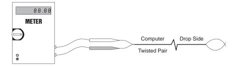
Figure 1 : Measuring Cable Impedance
