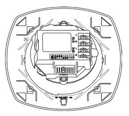
Adjust candela setting by turning dial with screwdriver. Candela selection is displayed on front of unit.
