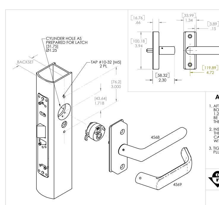
**HUB MUST BE** ON DIAMOND FOR PROPER INSTALLATION.
