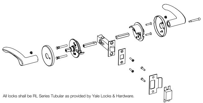
Locks shall have an interlocking tubular chassis and latchbolt. Chassis mounting screws shall be accessible only when the levers and roses are removed.
