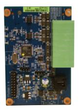
Honeywell's 4232CBM Connected Building Module is designed to support VISTA security panels with a variety of Honeywell and third-party hardware and software products.
