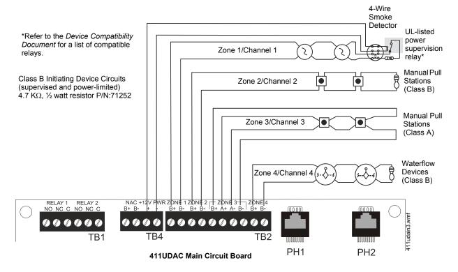
Figure 2.5 Wiring Initiating Device Circuits
