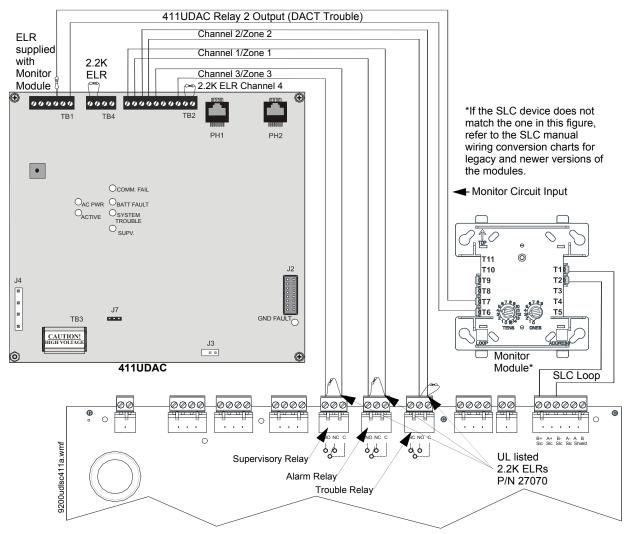
Addressable FACP (must be UL-listed for Central Station Service and Remote Signaling Service)
