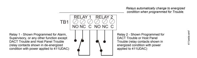
Figure 2.8 Programmable Relay
