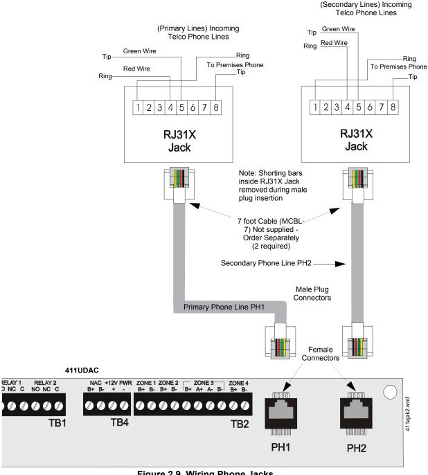
Figure 2.9 Wiring Phone Jacks
