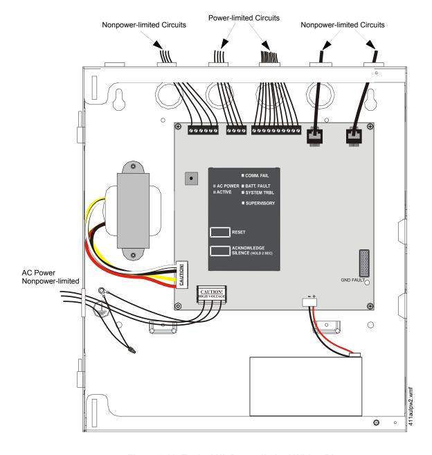
Figure 2.11 Typical UL Power-limited Wiring Diagram
