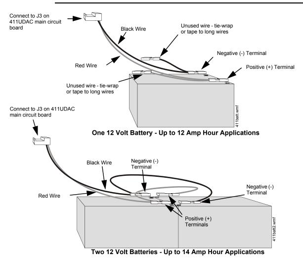
Figure 2.4 Battery Cable Connections
