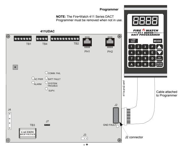
Figure 2.10 Programmer Connection to 411UDAC
