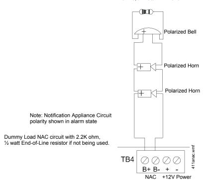
**Figure 2.7 Notification Appliance Circuit Connections**
