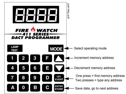
Address entry keys are 0 to 9. Data entry keys are 0 to 9 and A to F.
