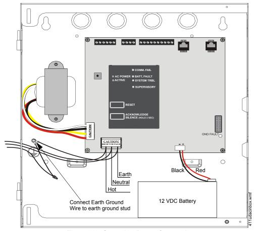
Figure 2.3 Operating Power Connections
