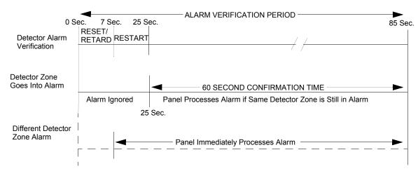
Figure 3.2 Verification Timing Diagram
