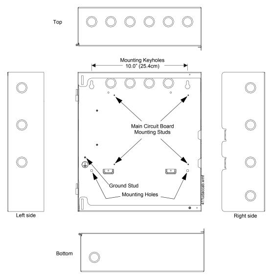
Figure 2.1 Cabinet Dimensions and Knockout Locations
