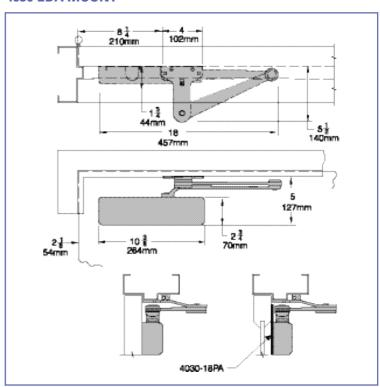
4030 closers ordered with EDA arms include 4030-201 FIFTH HOLE SPACER to support the shoe.
