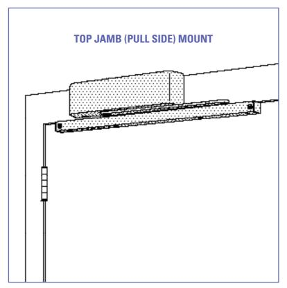
► Standard 4020T series closer is shipped with standard arm, standard track, track roller, standard plastic cover, and self reaming and tapping screws. See 4020T Series pages 21 & 22 for options.
