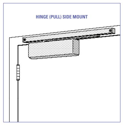
The 4010T SMOOTHEE® is LCN's best performing heavy duty track closer designed specifically for interior doors in institutional and other rugged high traffic applications.
