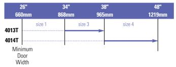
\*\*Note: Using this closer on double-egress doors and frames requires the closer to be ordered with a "DE" suffix (i.e., 4014T DE). Standard "DE" option will accommodate pull side reveals up to 3 5/16". For deeper reveals, consult factory.
