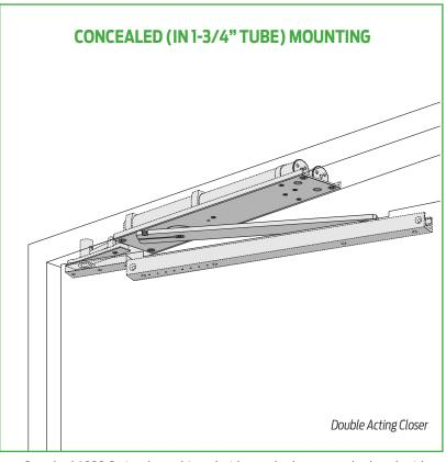
The concealed 6030 Series PACER® is a heavy duty, double acting closer designed to fit in a narrow, minimum 1-3/4" header. The single lever arm and roller assembly provides smooth, quiet door control and the choice of finishes and track functions meet virtually all architectural requirements. Installation at left illustrated with center pivot set (not included).
