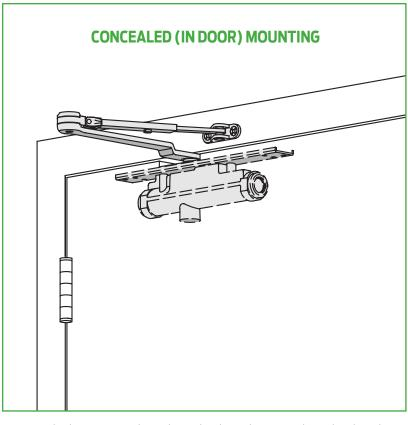
The concealed 3030 Series is designed to mount in a 1-3/4" interior door. The double lever arm provides superior door control and the choice of finishes and arm functions meet virtually all architectural requirements.
