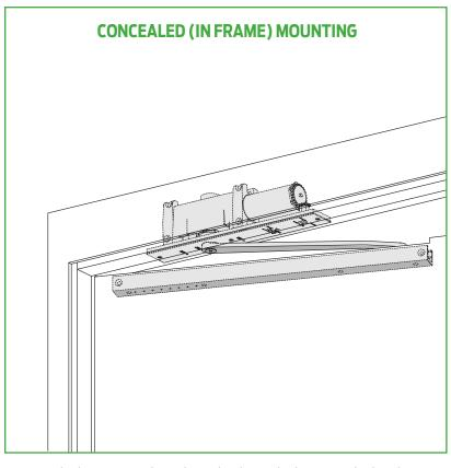
The concealed 2010 Series is a heavy duty closer designed to provide complete concealment. The single lever arm and roller assembly provide smooth, quiet door control and the choice of finishes and track functions meet virtually all architectural requirements.
