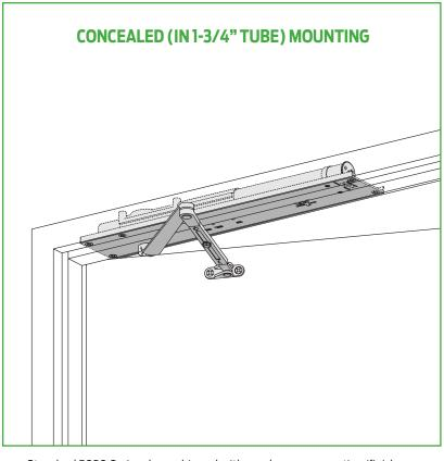
The concealed 5030 Series PACER® is a heavy duty closer designed to fit in a narrow, minimum 1-3/4" aluminum transom. The double lever arm provides superior door control and the choice of finishes and arm functions meet virtually all architectural requirements.
