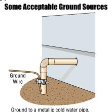
**IMPORTANT:** Ground wire shown without safety protection for clarity. Make sure ground wire is protected from being touched or electrical shock could occur!
