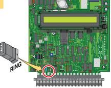
The PC programmable telephone entry system has two relays on the circuit board, all of which are programmable for any function required. These relays are designated as Relay 1 (R 1), and Relay 2 (R 2).
