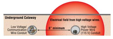
**DO NOT** run high voltage (115 V) power lines and low voltage/communication lines in the same conduit. These should be in separate conduits at least six (6) inches apart. Be sure that all phone line wiring is twisted and completely isolated from ground.
