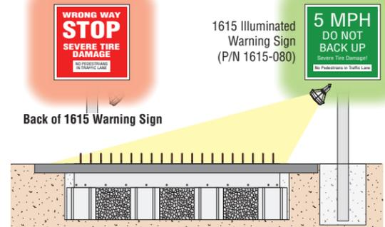
Additional lighting, warning signs and pavement markings can be used to increase awareness for potential danger and to separate pedestrians from vehicular traffic.
