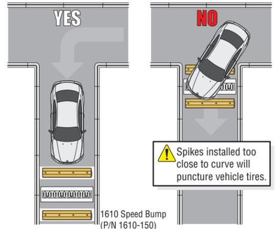
Traffic spikes must be installed in flat-leveled concrete avoiding bumps or dips including uphill or downhill slopes minimizing the possibility of water draining into the spike assembly.
