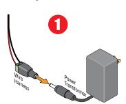
Un-plug power transformer from wire harness.
