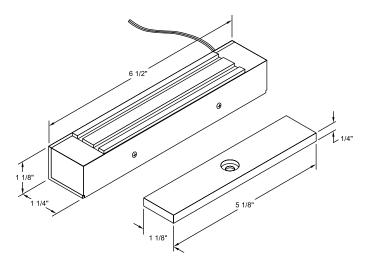
Figure 2. 1583 EMLock® with AC transformer, rectifier, key switch and LED (green when locked, red when unlocked)
