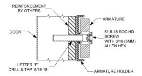
Figure 2C – REINFORCED ALUMINUM OR HOLLOW METAL DOOR
