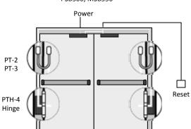
Pair of doors with two locks and required TC-3 cable for power and slave operation Sense Bar Trigger Non-Latching PSB560, MSB550
