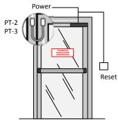
Sense Bar Trigger Non-Latching PSB560, MSB550
