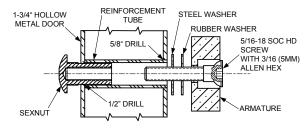
FIG. 2A HOLLOW METAL DOOR From Sexnut side of door, drill exactly 1/2" hole thru one metal thickness only. From Armature side of door, drill 5/8" hole to insert reinforcement tube. Press in sexnut and reinforcement tube all the way and mount armature to door using hardware provided per Figure 2B.
