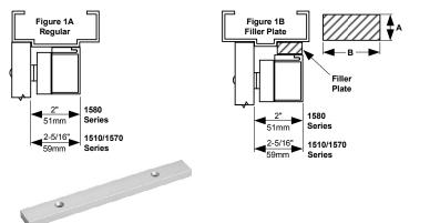
FILLER PLATES: For extension of the stop to provide a proper mounting surface on the underside of the header. See Figure 1B.
