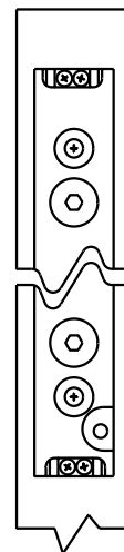
FIG. F 006-001-03 Even shear tabs ARMATURE TOP VIEW For locks with bond sensor
