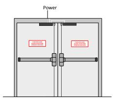
A pair of doors requires the 1511T Pushing either door triggers the delayed release of both doors.
