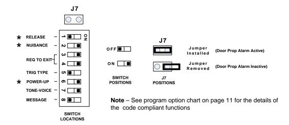
**RELEASE TIME\*** – The Release time can be selectable for 15 or 30 seconds. The Nuisance Delay time period is included in the door release cycle and it will not increase or decrease the "total time to unlock" once the ExitCheck<sup>TM</sup> is activated.
