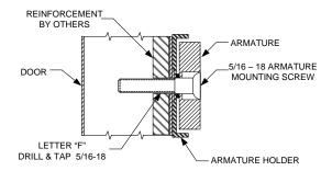
Figure 2C – REINFORCED ALUMINUM OR HOLLOW METAL DOOR
