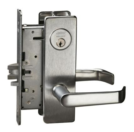
The Corbin Russwin ML2000 Series Mortise Lock, is an ANSI/BHMA A156.13 Series 1000 Grade 1 mechanical mortise lock. It has a reversible latch with stainless steel insert and an independent non-handed stainless steel deadlatch.
