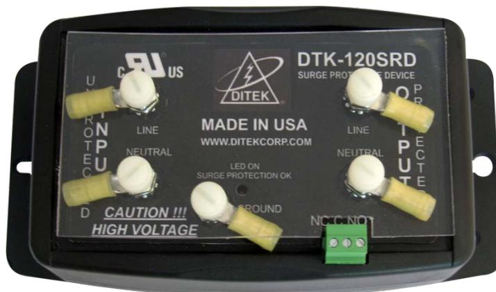
DITEK's DTK-120SRD protects 120V power on electrical circuits and control panels and has Dry Contacts for remote notification of surge protection status. The hybrid series design provides maximum critical load protection, with EMI/RFI filtering. The 120SRD is ideal for use in UL Listed control panels where a UL Recognized Component is required. Use DITEK's DTK-TSS4D when a UL Listed series surge protector with Dry Contacts is required.
