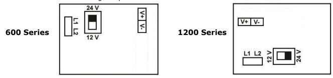
A terminal block is provided for wiring the maglock to the power supply.
