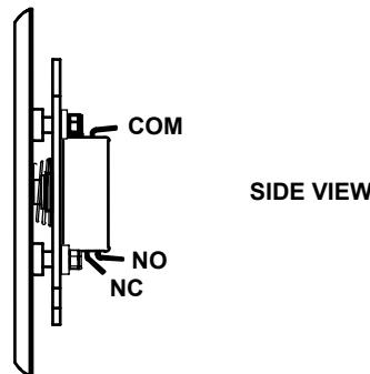
2. Finger-tighten the enclosed hex-head screws into the electrical enclosure.
