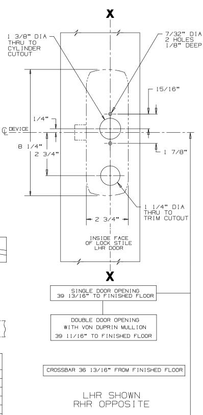
NOTE; MOUNTING HOLES TO BE PREPARED AT INSTALLATION ON DOOR.
