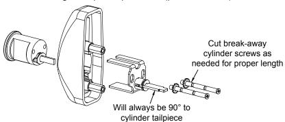
6. GO BACK AND FOLLOW EXIT DEVICE INSTRUCTION STEPS up to, but not including ASSEMBLE DEVICE TO DOOR. Trim must be installed BEFORE device is assembled to door.
