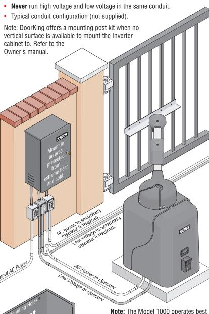
**Note:** The Model 1000 operates best when it can be installed as physically close as possible to the equipment that it will operate during power outages. This reduces line loss.
